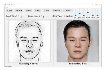
Fig. 8. A screenshot of our shadow-guided sketching interface (Left) for facial image synthesis (Right). The sliders at the up-right corner can be used to control the degree of interpolation between an input sketch and a refined version after manifold project for individual components.
