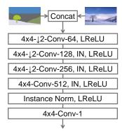
Figure 13: Our discriminator design largely follows that in the pix2pixHD [40]. It takes the concatenation the segmentation map and the image as input. It is based on the Patch-GAN [20]. Hence, the last layer of the discriminator is a convolutional layer.
