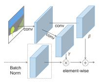
Figure 2: In SPADE, the mask is first projected onto an embedding space, and then convolved to produce the modulation parameters  $\gamma$  and  $\beta$ . Unlike prior conditional normalization methods,  $\gamma$  and  $\beta$  are not vectors, but tensors with spatial dimensions. The produced  $\gamma$  and  $\beta$  are multiplied and added to the normalized activation element-wise.
