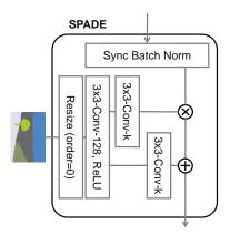
Figure 10: SPADE Design. The term 3x3-Conv-k denotes a 3-by-3 convolutional layer with k convolutional filters. The segmentation map is resized to match the resolution of the corresponding feature map using nearest-neighbor downsampling.
