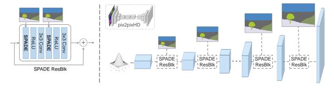
Figure 4: In the SPADE generator, each normalization layer uses the segmentation mask to modulate the layer activations. (*left*) Structure of one residual block with SPADE. (*right*) The generator contains a series of SPADE residual blocks with upsampling layers. Our architecture achieves better performance with a smaller number of parameters by removing the downsampling layers of leading image-to-image translation networks (pix2pixHD [40]).
